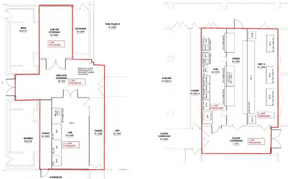
Figure 7: Cleanroom Pressurization Plan -Hybrid MSC
