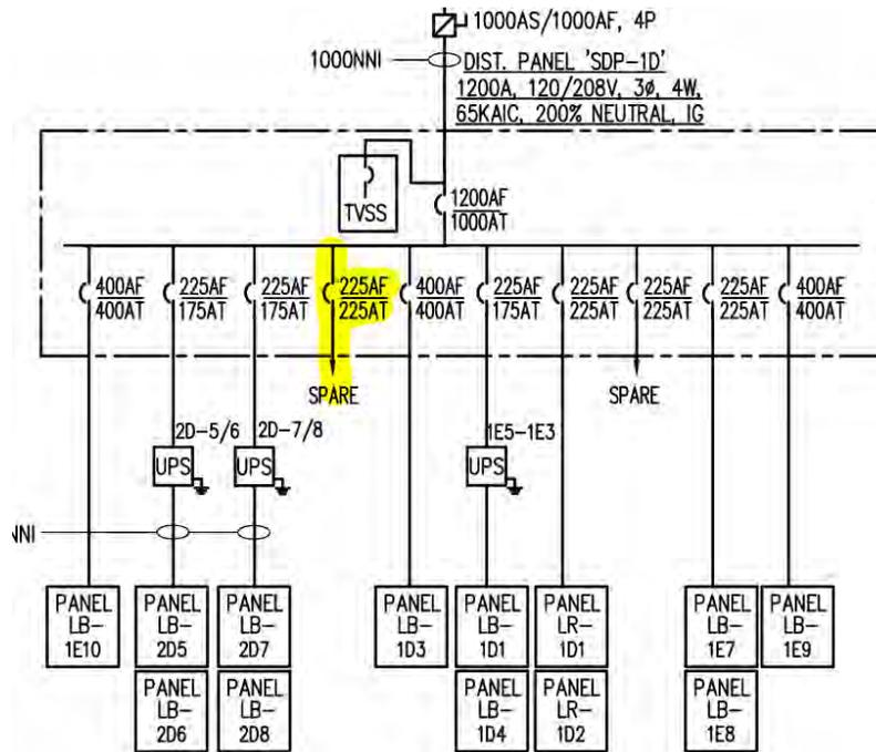
**Figure 15: One-line Diagram of Power Distribution**
