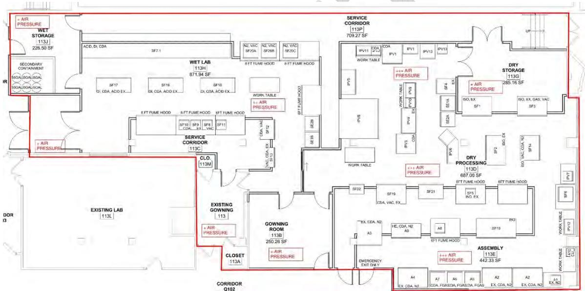
Figure 5: Cleanroom Pressurization Plan
