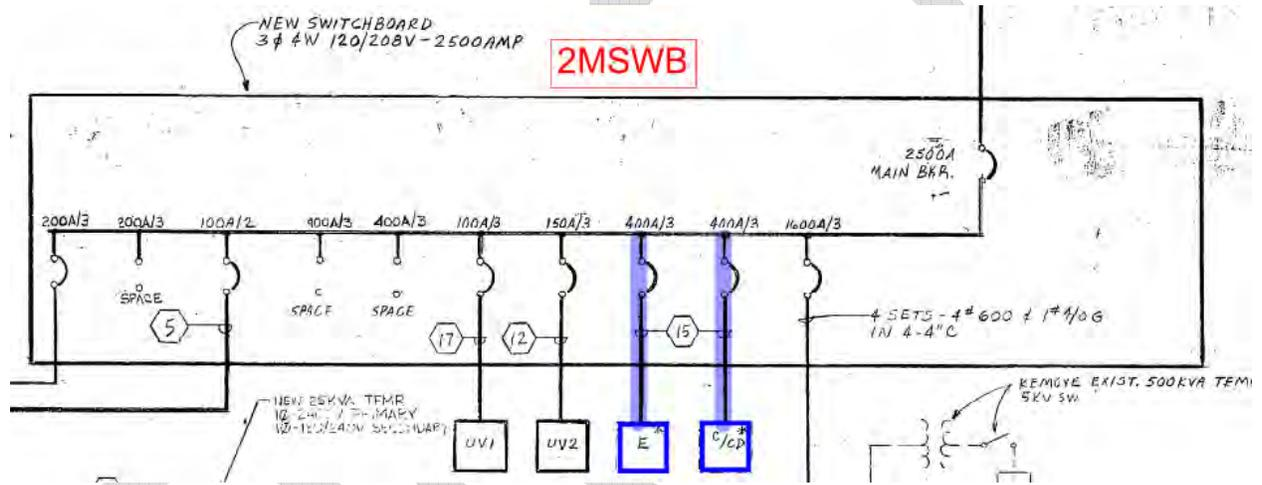
Figure 12b: One-line Diagram of Panelboard Feeds
