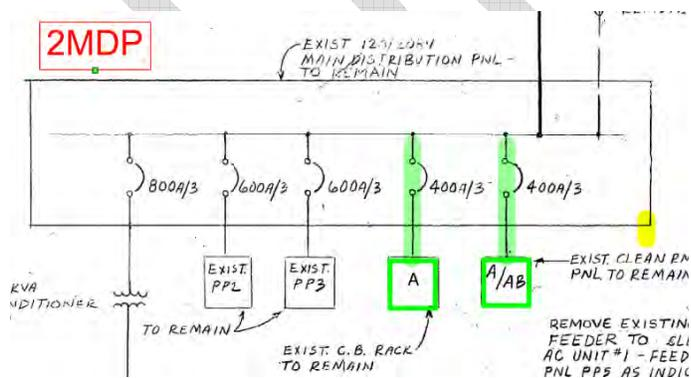
Figure 12c: One-line Diagram of Panelboard Feeds
