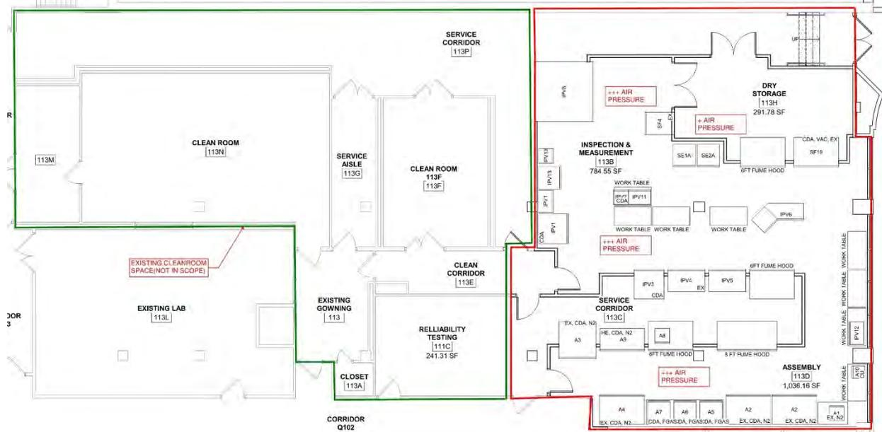
Figure 6: Cleanroom Pressurization Plan -Hybrid EEW
