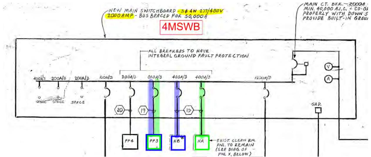
Figure 12a: One-line Diagram of Panelboard Feeds
