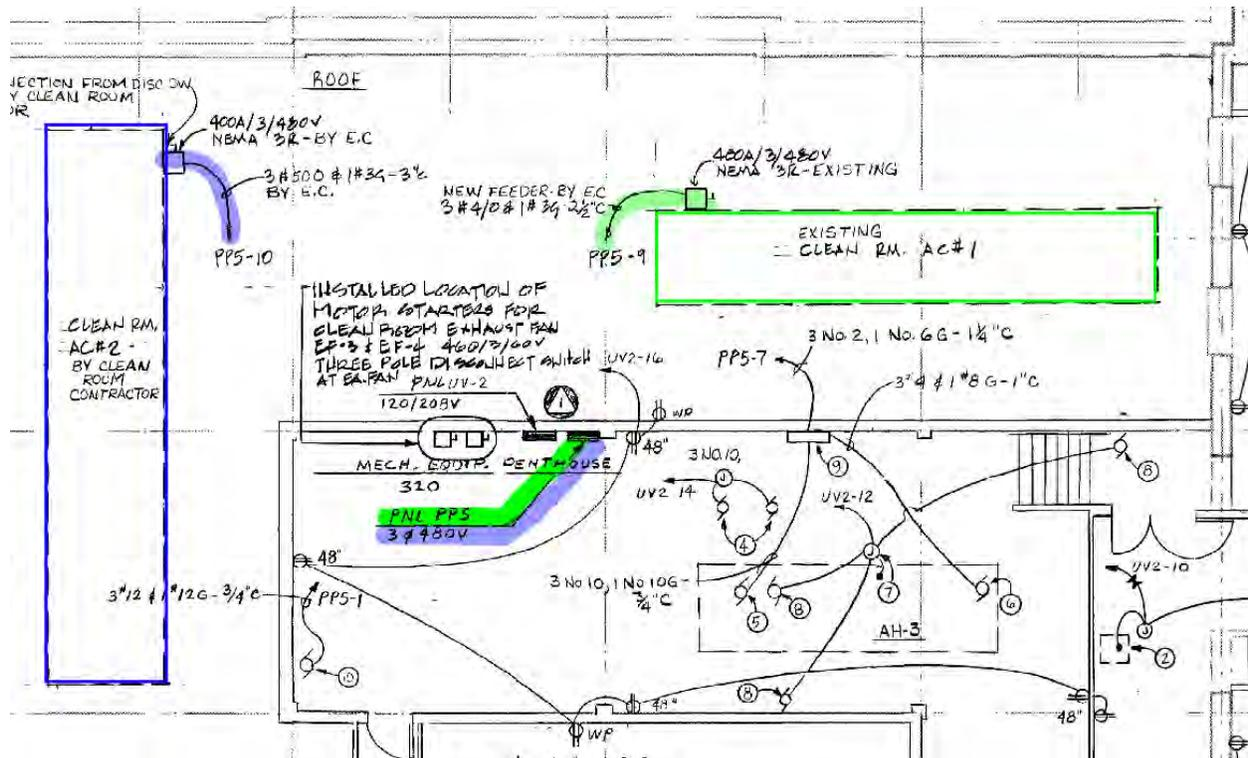
**Figure 13: Rooftop HVAC Equipment Power Supply Plan**
