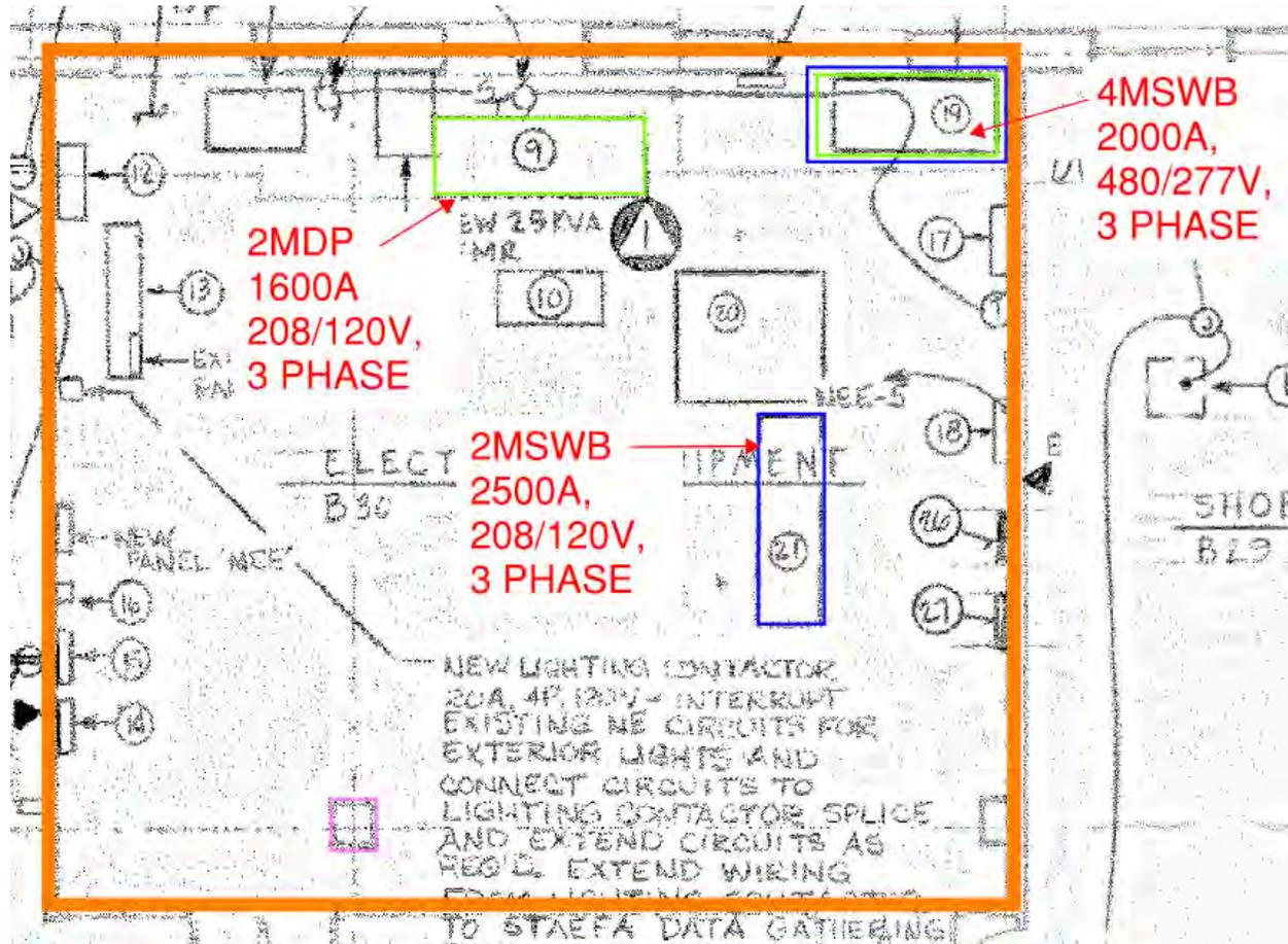
Figure 11: Main Electrical Room Distribution Switchboard Plan
