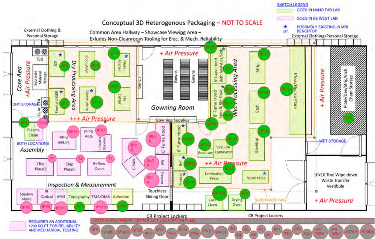
Figure 4: Early Study Partial Equipment Distribution Layout
