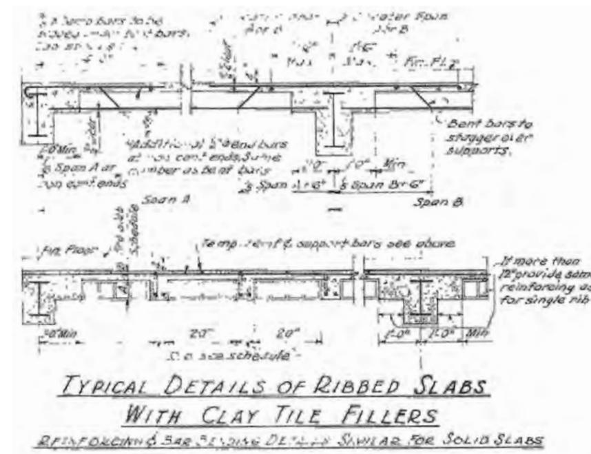
Typical Ribbed Slab with Clay Tile Filler Detail
