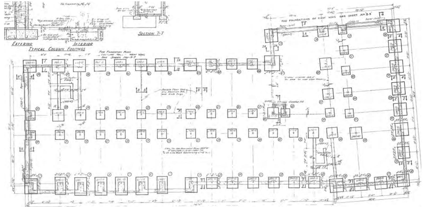
Typical Foundation Configuration, as Shown on Existing Drawing S-1
