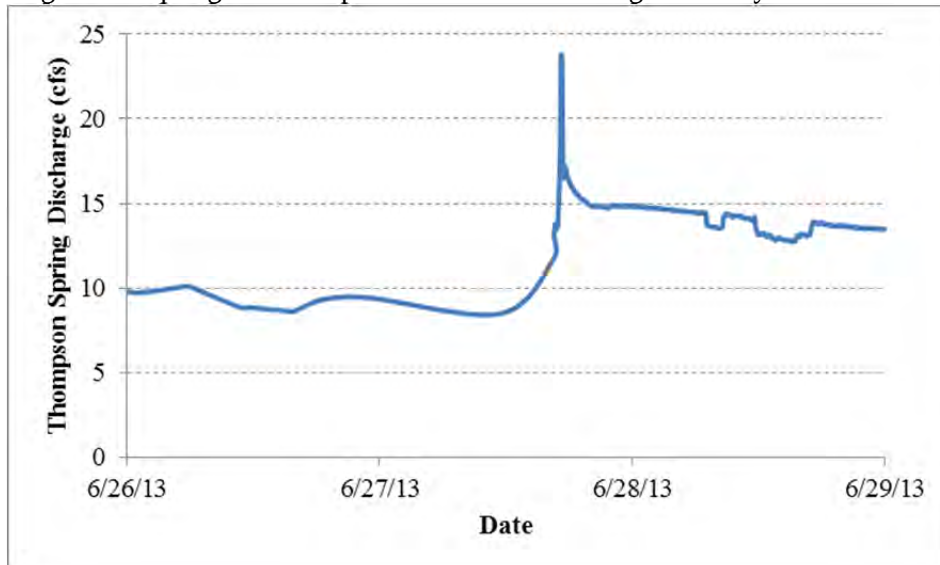
Figure 56. Spring Flow Response Due to a Large High Intensity Rainfall Event
